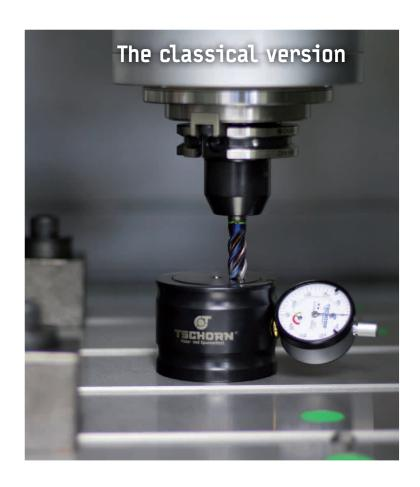
To determine the position of workpiece surfaces or tool lengths in Z-direction at milling machines or turning lathes. The zero setter is placed on the workpiece. The spindle has to be moved carefully onto the tracer until the dial gauge indicates "0". The reference dimension 50 mm to the workpiece has been reached. A safety spring range of max. 2 mm is included.
