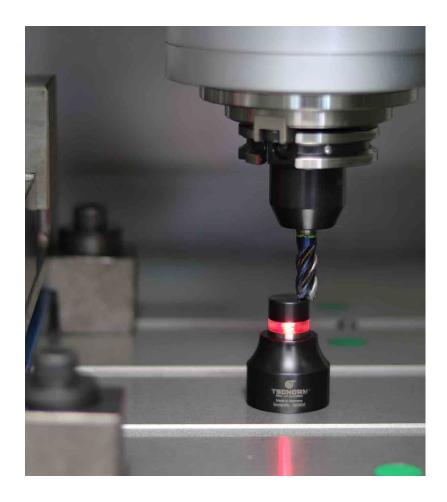
To determine the position of workpiece surfaces or tool lengths in Z-direction at milling machines or turning lathes. The zero setter is placed on the workpiece. The spindle has to be moved carefully onto the tracer until the dial gauge indicates "0". The reference dimension 50 mm to the workpiece has been reached. A safety spring range of max. 2 mm is included.
