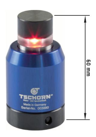
To determine the position of workpiece surfaces or tool lengths in Z-direction at milling machines or lathes. The zero setter is placed on the workpiece. The spindle has to be moved carefully onto the tracer until the dial gauge indicates "O". The reference dimension 60 mm to the workpiece has been reached. A safety spring range of max. 2 mm is included.
