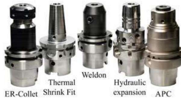
Fig. 1 Examples of the investigated tool holder systems
