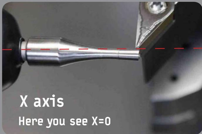
Without any further calculation, you measure your tools to the centre of the spindle, respectively  $X=0$ .
