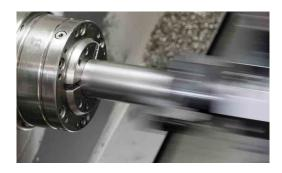
Pull the bar to the desired position in Z.
