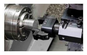
Position the bar gripper in Z axis in front of the bar.
