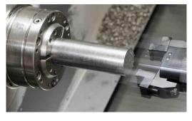
Move the bar puller in Z direction off the bar and start machining.
